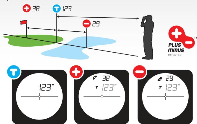
For Example a MAIN TARGET distance can be measured to the front of the green and the EASY 800 operates like a standard Laser Rangefinder.
